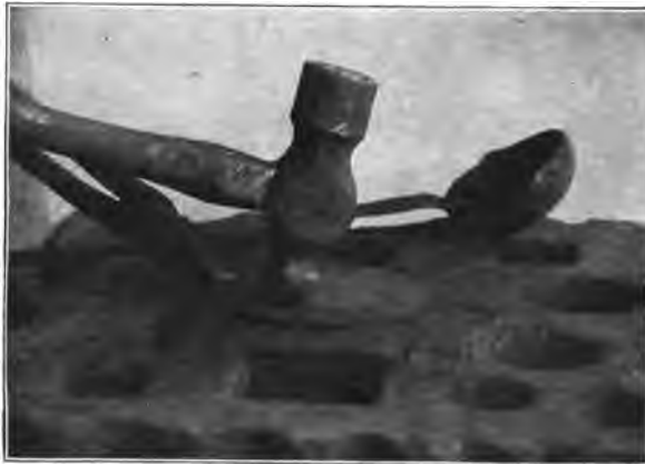
Fig. 85. Method of Rounding Ladle Bowl
